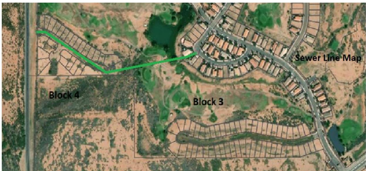
\*Sewer line depicted in green. The sewer line goes through Block 4; sewer is available to the east of Block 3.
