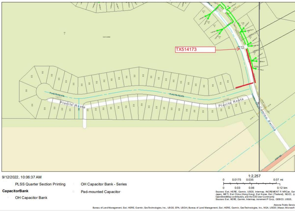
\*Block 3 Electric is available at the east end of the block depicted by the red line. The power in this area is underground.
