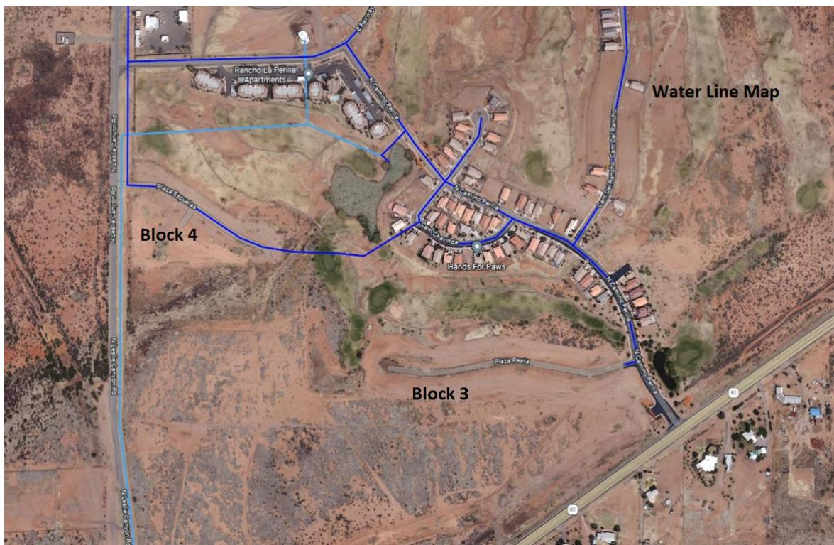
\*Water line depicted in blue. The water line goes through Block 4; water is available to the east of Block 3.
