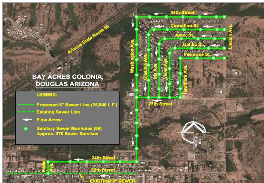
Figure 2.6: System Layout, Gravity Sewer System (Alternative 2)
